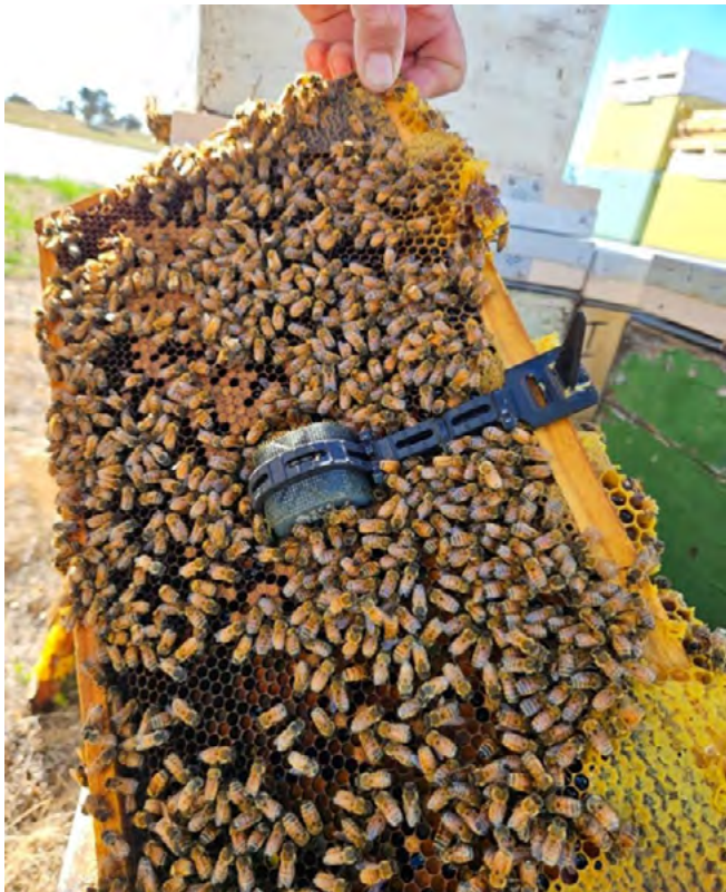
Above: LB AgTech's in-hive sensor installed between the centre frames of the hive. Photo credit LB Agtech.
