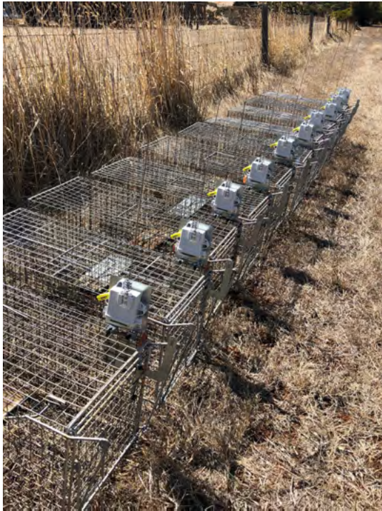
Cage traps (left) fitted with Celium sensors ready for deployment and a Celium hub (right) which communicates with trap sensors and reports status.
